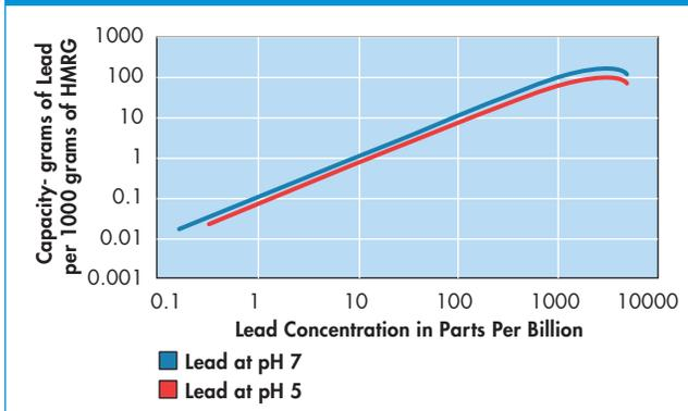
Adsorption isotherms for lead between pH 5 and 7 are nearly identical.
