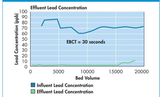
Lead removal by MetSorb® HMRG adsorbent in column test; 30 seconds EBCT.
