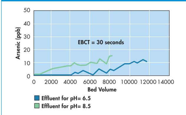
Testing was done under the conditions specified by the NSF Standard 53 for Arsenic. Results at a pH of 6.5 and a pH of 8.5 are shown in the graph above.
