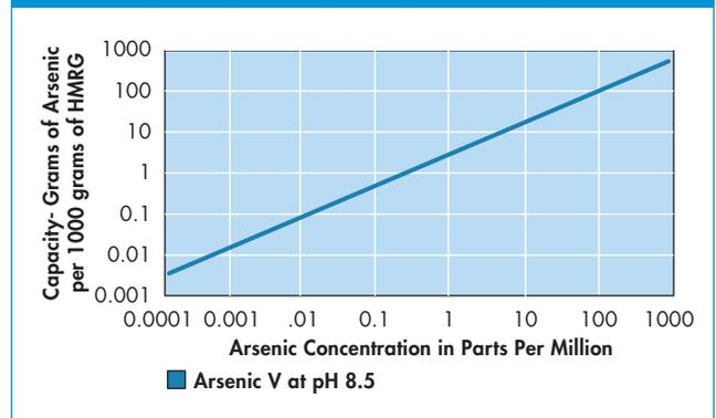
The above graph shows the adsorption isotherm for Arsenic V at pH 8.5.
