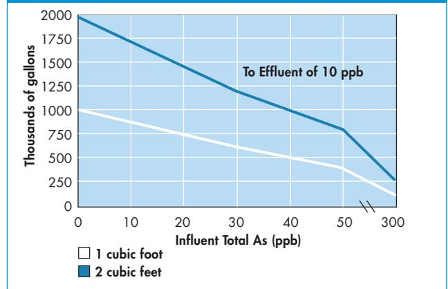
Treatment capacity as a function of tank size.
