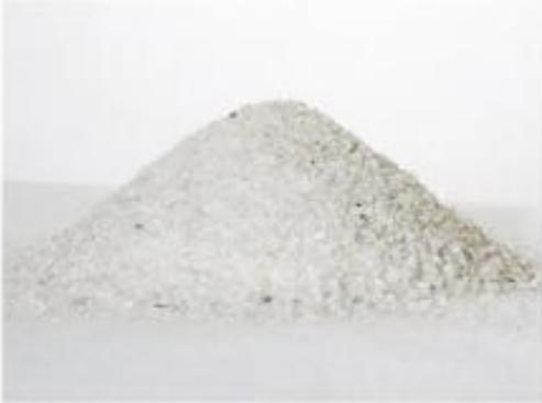
Puri-Cal™ brand water treatment calcite is a safe, easy to use, natural product from high purity Pacific Northwest Limestone. It is specially selected and sized to optimally adjust pH in potable water systems. When used in accordance with standard water treatment practices it will gently and effectively adjust the pH of your water and help minimize
