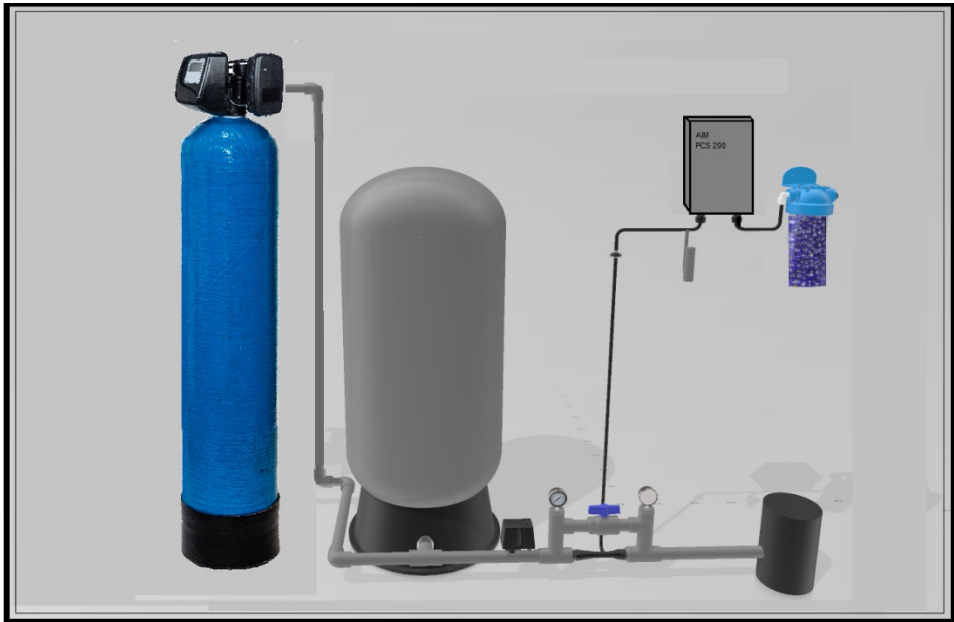
Figure 2. Typical well application w/EOG filter
